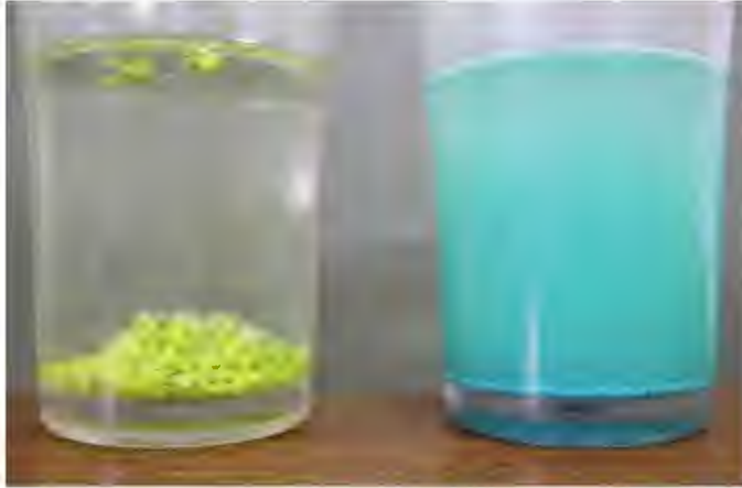
Figure 5: AgriCote (right) dissolves much quicker in water than other coating formulations built with Talc, instead of lime. This results in quicker establishment. Photo taken 3 hrs post coating in water suspension.
